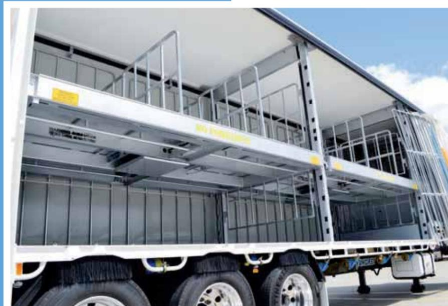
can also save on shipping costs for the client. "Another key aspect is that the system is able to reduce the amount time wasted in changing the deck position. Some companies won't allow you to change the height of the decks on site, so that means the operator must go back to a depot and
